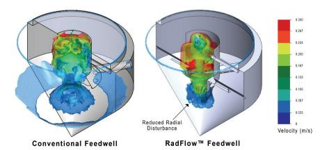
The CFD schematic (image to the left) indicates velocity isoprofiles for a conventional feedwel installed in a clarifier verses a RadFlowTM feedwell.
